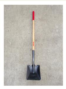
**Square blade shovels:** Square blade shovels are used for scooping loose materials, such as dirt, mulch, or sand.
