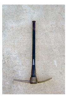
A pick mattock has a metal head with a pointed end (pick), used for breaking up hard surfaces or objects, and a flat end (adze), used for breaking up soil and prying. Pick mattocks can be used to dig holes and trenches, "hand-till" soil, and break up hard surfaces or objects, such as concrete or rocks.
