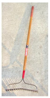
A bow rake has a long handle with stiff metal tines. Bow rakes can be used to evenly spread loose materials, such as soil, sand, and mulch.
