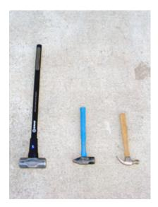
Hammers are available in various weights and shapes specific to their intended task. Some hammers are used for driving nails, while heavier hammers (such as <u>sledgehammers</u>) are used for breaking concrete or driving stakes.
