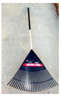
A leaf rake has a long handle with flexible metal or plastic tines. Leaf rakes can be used to gather or spread loose materials, such as leaves, soil, sand, and mulch.
