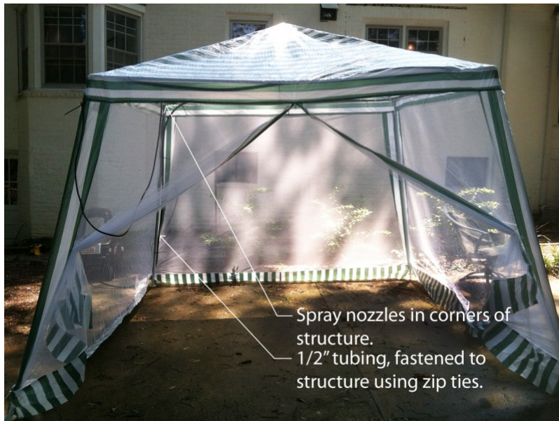
Figure 4. Completed Misting Station
