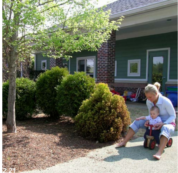
2.21 Toddler pathway concrete base is surfaced with a thin coat of poured-in-place soft surfacing. "Watch out, here we come!"
