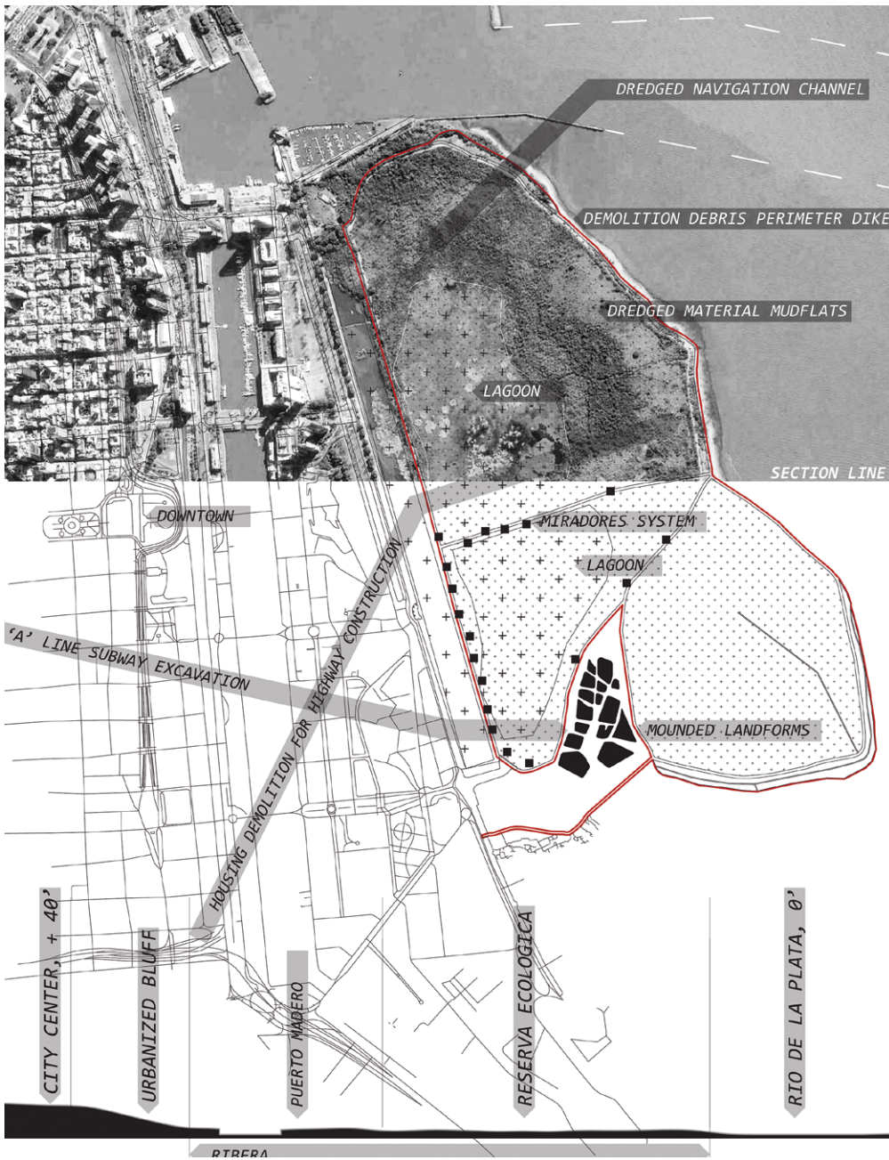
Figure 7 Plan and section composite. This aerial and section cut show the ribera and its landscapes of material reuse in relation to the bluff and historical core of Buenos Aires.
