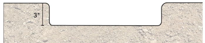
1A. Excavate soil a minimum of 3" for a 2" thick stone
