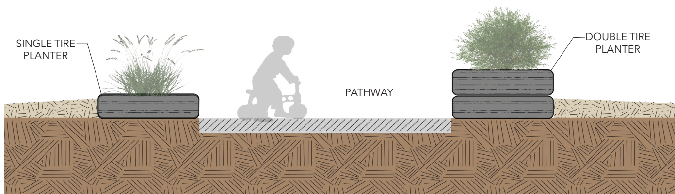
Cross section of single and double tire planters used to edge a wheeled toy, primary pathway.
